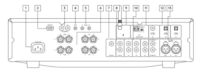
**1. AC power socket** - Once you have completed all connections to the amplifier, plug the AC power cable into an appropriate mains socket then switch on. Your amplifier is now ready for use.
