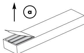
b) If necessary, remove used batteries and insert new ones correctly as shown by the diagram in the battery compartment.
