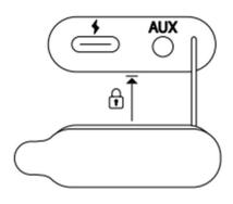
On the back side there is a plastic cover with some technical connections behind. Connect the USB-C jack on the left with the included power supply unit.
