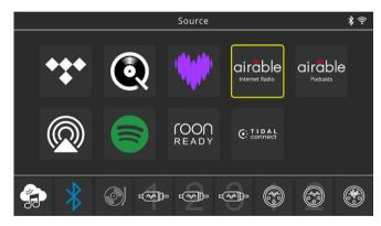
The corresponding sources can be selected and configured by swiping left or right on the display or by using the arrow keys on the remote control.
