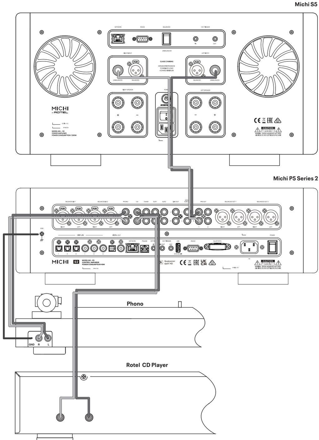
**Figure 5: Balanced (XLR) Input and Output Connections**
